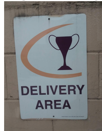
Picture Taken 12-12-18 Originally Printed 1-16-15 Black is now just starting to fade to a reddish brown tint
